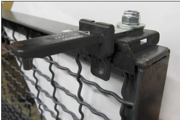
Install key on the door of the enclosure so that it aligns with the switch on the side panel.
