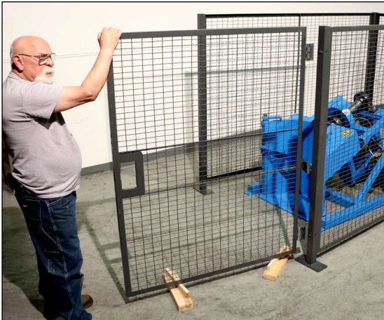
Use spacer blocks (not provided) to support door panel during set up.
