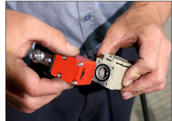
If necessary, reverse orientation of switch. . .
